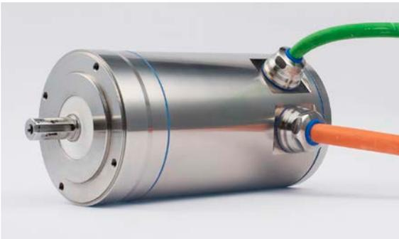
**Figure 6:** Motor H does not have any metal to metal joints. Instead, all joints are mated with gaskets. The gaskets are bright blue in color to contrast against food products.
