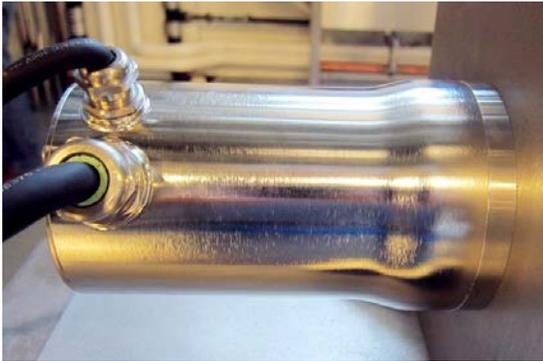
**Figure 5:** Motor C has metal to metal joints at both ends of the motor body. The end cover joint is secured with six screws as seen in Figure 2.
