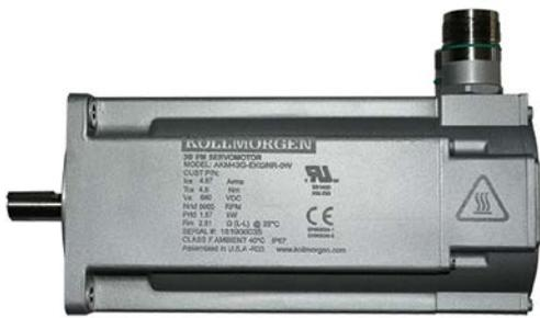
**Figure 1:** Motor W has an etched label covered with paint. The etching process creates a rough uneven surface that can create niches where bacteria and food product may be harbored.
