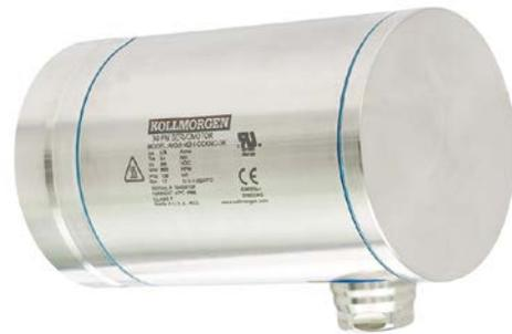
**Figure 3:** Motor H features an annealed label with a 32  $\mu$ -inch surface finish. Unlike etching, the annealed label preserves the metal's surface finish. This smooth label was designed to avoid trapping bacteria or food.
